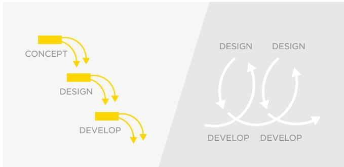
**Figure 7. Waterfall (left) versus Agile Design (right) Methodologies**
